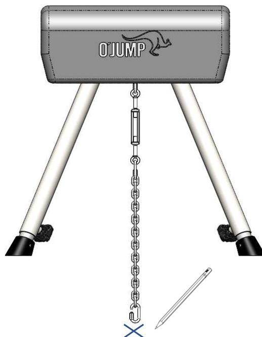
2. Drill all the holes using a drill bit appropriate for your floor. Place the fixations in the holes. They should not be higher than the ground.
